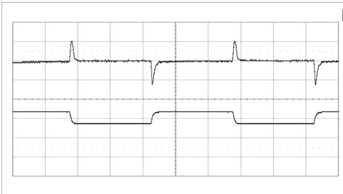
Output voltage response to load current step change (1.5–4.5–1.5 A) at V_I = 12\text{ V} , C_O = 3 \times 100\ \mu\text{F} + 270\ \mu\text{F}/10\text{m}\Omega . Default compensation settings. Scale: 20 mV/div, 5 A/div, 100 \mu\text{s} /div.
